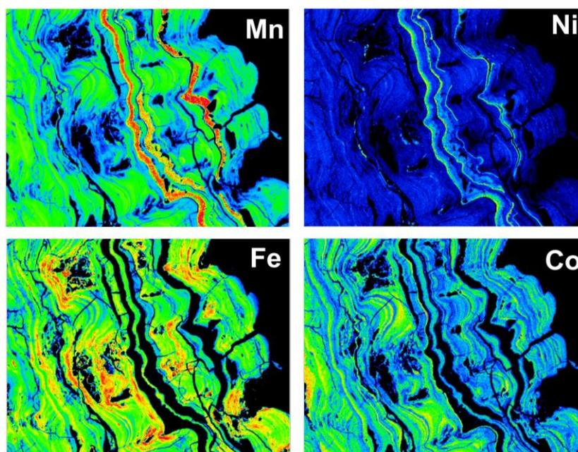
**Figure 10.** Electron probe microanalyzer (EPMA) strategic and CRMs mapping obtained on a thin section of a Fe-Mn crust (Marino, 2020).
