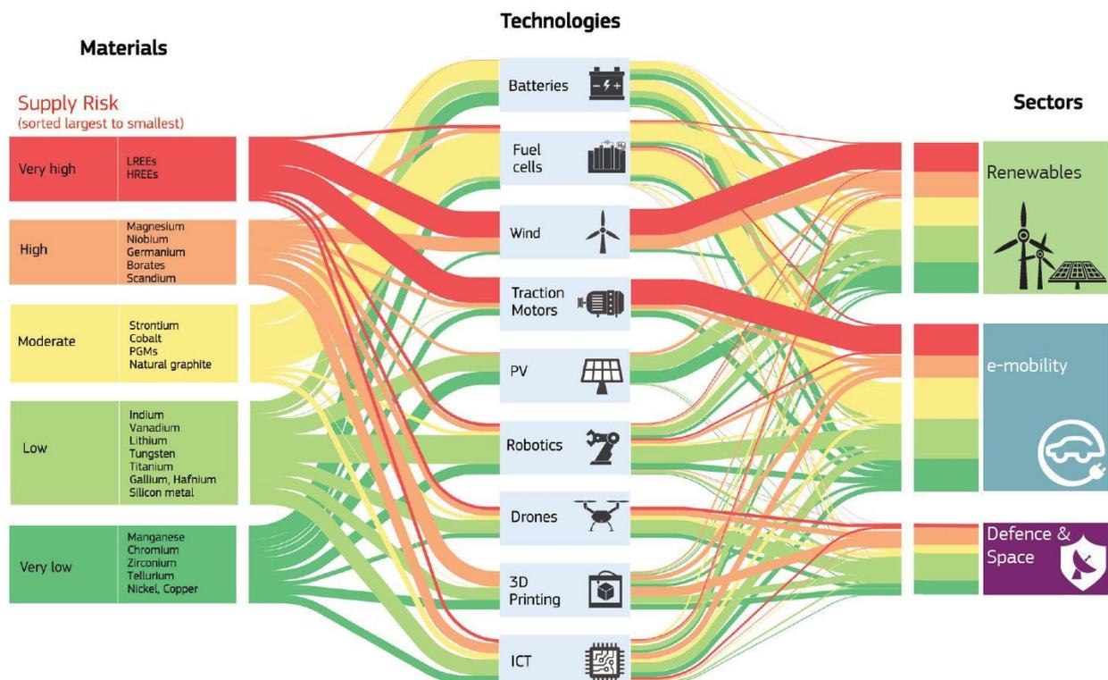
**Figure 2.** Schematic presentation of different CRMs and their uses in high tech and defence industry (Bobba et al., 2020).
