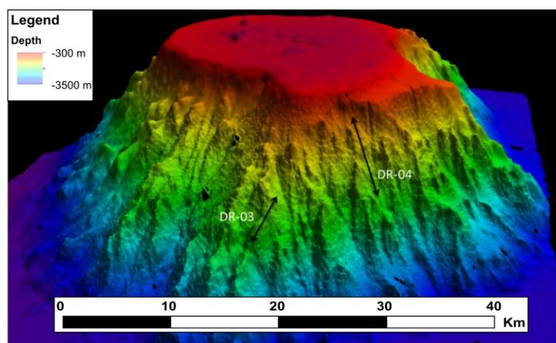
**Figure 9.** A) 3D bathymetric model representing the guyot-type Echo Seamount in the CISP with location of dredge stations (DR-03 and DR-04). Abundant pavements of ferromanganese crusts were recovered on the slopes. *DRAGO0511* Expedition.
