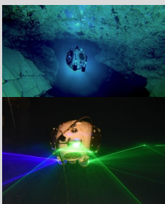
UNEXMIN developed an autonomous device specially designed for flooded mines and equipped with sonars, digital cameras, scanners and lasers, a water sampler, a sub-bottom profiler and multispectral cameras (with courtesy by UMEXMIN).
